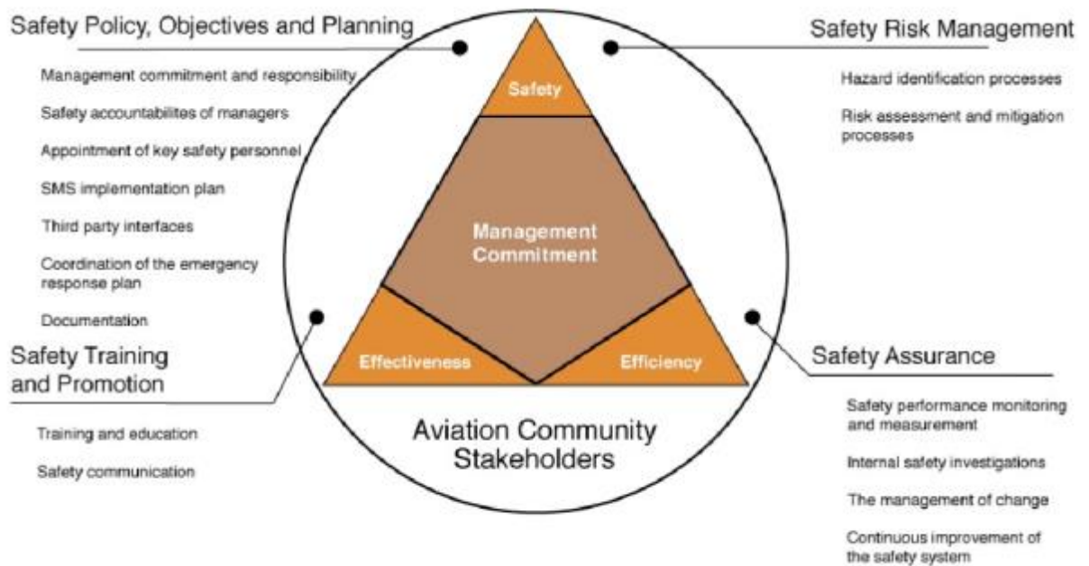
Figure 26: Key aspects of a safety management system as required by the Australian Civil Aviation Safety Authority (CASA) [191]
